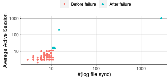
Figure 1: Joint distribution of the Average Active Session (an SLI of the Oracle database) and the number of log file sync waiting events within 2 hours. Each data point represents the two metrics’ values at the same timestamp.
