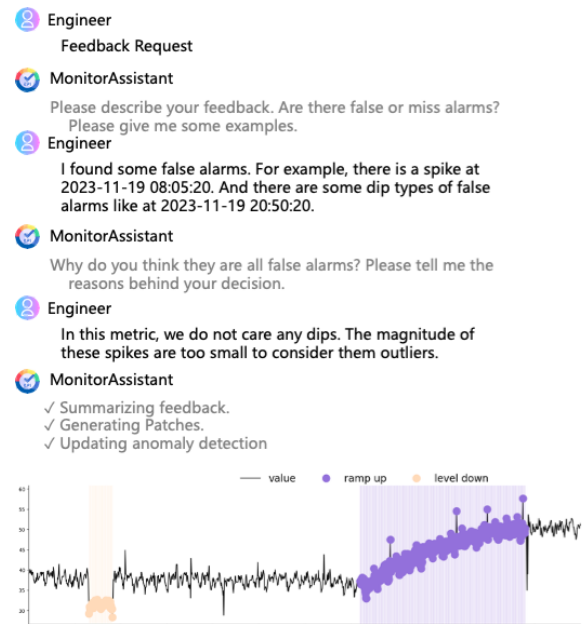
Figure 11: Case for feedback loop. Ramp up anomalies are marked by purple, level shift down anomalies are marked by yellow.
