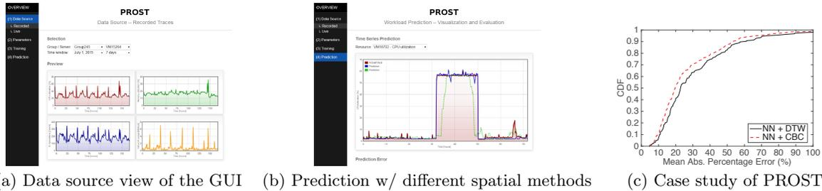
**Figure 2: Data source view of the GUI to select the servers of interest, showing a preview of the selected VM’s resource utilization traces and prediction of using different spatial methods, and a case study of PROST on predicting usage series at private datacenters.**
