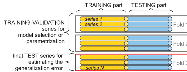
Fig. 9. Estimating the generalization performance of the technique(s) across multiple individual (but related) data streams by cross-validating the data streams.
