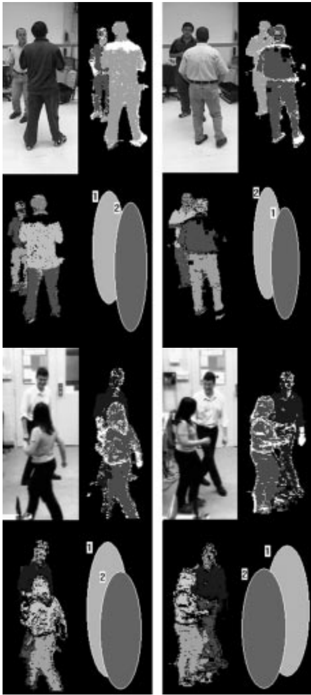
Fig. 11. Example results. Top left: original image. Top right: people segmentation. Bottom left: blob segmentation. Bottom right: constructed occlusion model.
