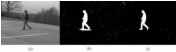
Fig. 4. (a) Original image. (b) Detection using (R, G, B) color space. (c) Detection using chromaticity coordinates (r, g) .
