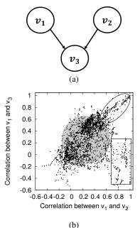
Figure 3: Effect of external factor. Even though a sensor  $v_3$  is called by both  $v_1$  and  $v_2$  in (a), the correlation between  $v_1$  and  $v_2$  can be high even when the correlation between  $v_1$  and  $v_3$  is low in the rectangle area of (b). The rectangle area is caused by the colocation of  $v_1$  and  $v_2$ .
