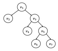
Figure 4: Natural trapping in the call graph. Due to the nature of downward sensor calls (from frontend to backend tier), when the random walker falls into the branch of  $v_3$ , the random walk cannot visit  $v_2$  until the next teleportation even if there is no sensor related to the given anomaly in  $v_4 \sim v_7$ .
