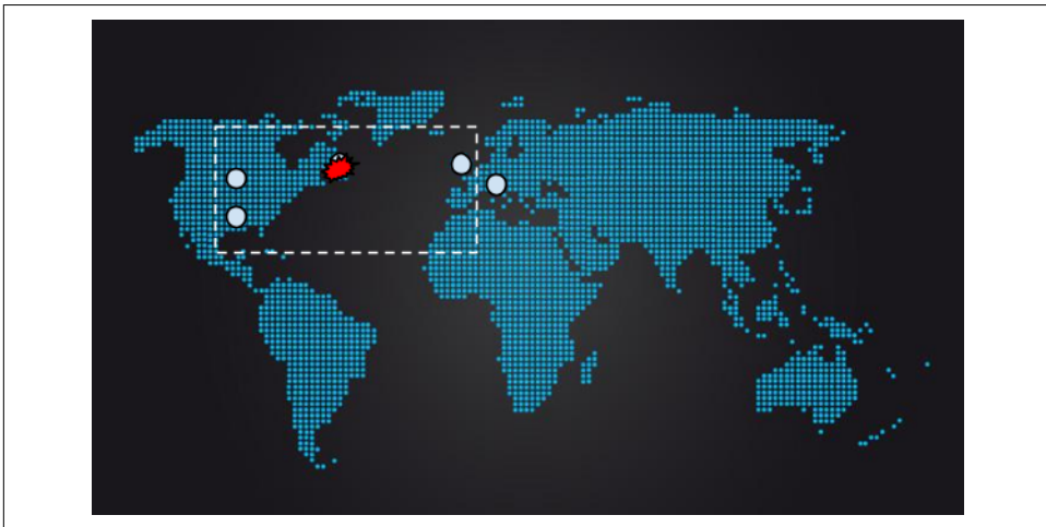
Figure 23-14. Loss of the link replica immediately leads to a longer RTT for any quorum
